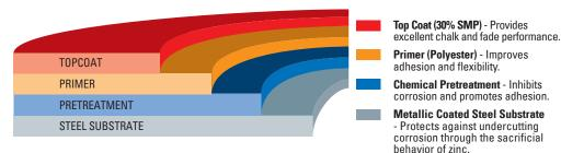
Coated steel, a pretreatment of chrome oxide is applied which also inhibits corrosion and promotes adhesion. Next, a primer, consisting of an epoxy modified polyester for improving adhesion and flexibility, is laid down. Lastly, the topcoat is used consisting of a 30% siliconized modified polyester (SMP) which minimizes chalk and fade.
